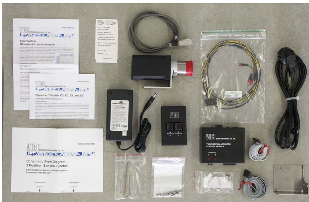
Figure 1. Contents of CS valve option kit, p/n 250.0024.
